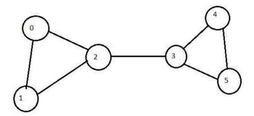
If the republic loose the path between 2 and 3 then the two system of planets will not be able to communicate with each other. Hence 2 and 3 are critical planets.
